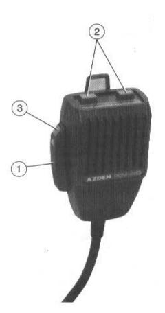
(1) Push—to—Talk Switch Lever To transmit, depress the Push—to—Talk (PTT) switch and speak slowly and clearly in your normal tone of voice with the microphone about two inches from your mouth. Depressing the PTT switch turns the TX indicator Light on the LCD, indicating that the transmitter is in operation.
