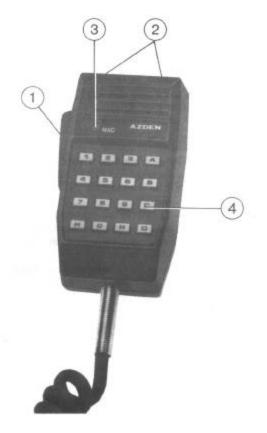
(1)To transmit, depress the Push—to—Talk (PTT) switch and speak slowly and clearly in your normal tone of voice with the microphone about two inches from your mouth. Depressing the PTT switch turns the TX indicator light on the LCD, indicating that the transmitter is in operation.
